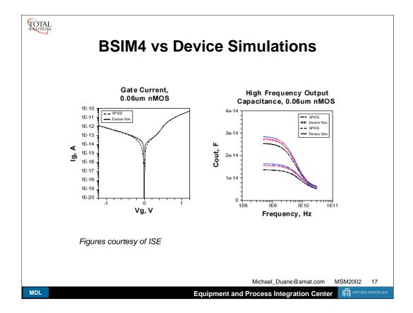
And these figures show how device simulators can reproduce deep submicron physics. A cynic might point out that I am just showing how a compact model can fit a device simulation, but there are equally good fits between silicon and TCAD not shown here.
