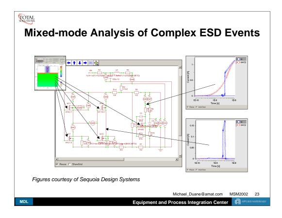
ESD is a special case worth highlighting. Here, I show a mixedmode simulation where an actual transistor is simulated in a device simulator while part of a conventional circuit simulation. This is necessary in cases where there is no compact model that describes the electrical behavior of the device in certain operating conditions.
