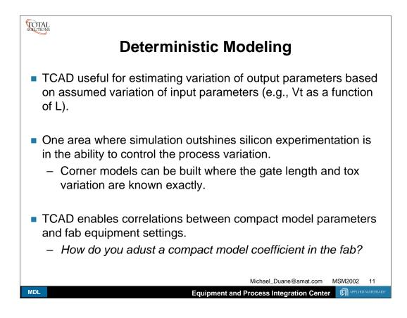
Along these same lines, simulation is good for generating realistic corner models. You can see how different Lgate control affects your circuit performance.
