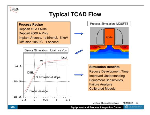
This slide shows the typical flow in TCAD simulation. Starting from a process recipe and knowledge of the layout, a structure is created via process simulation. This structure feeds directly into the device simulator, which produces IV or CV curves.
