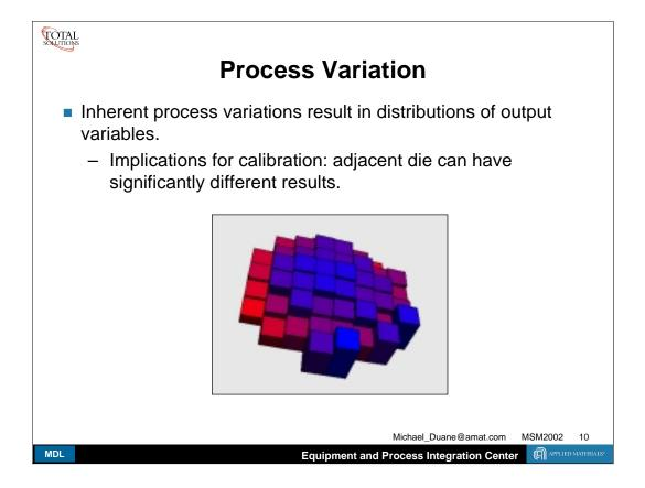
When calibrating TCAD, you have to know your structure *exactly*, or else simulate a range of input variables and see if your measured results fall with the simulated output range.
