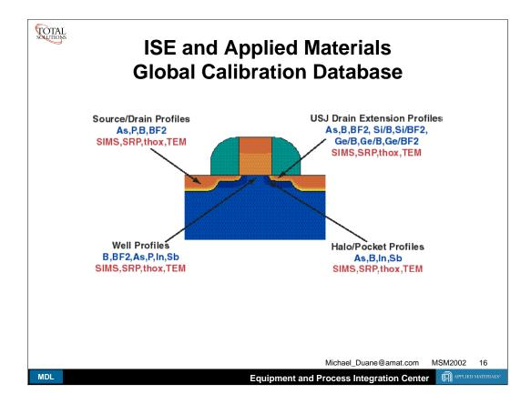
The figure above shows some of the areas where the calibration project with ISE initially focused on. There has also been work on oxidation modeling. Literally hundreds of SIMS have been taken. This work is ongoing.
